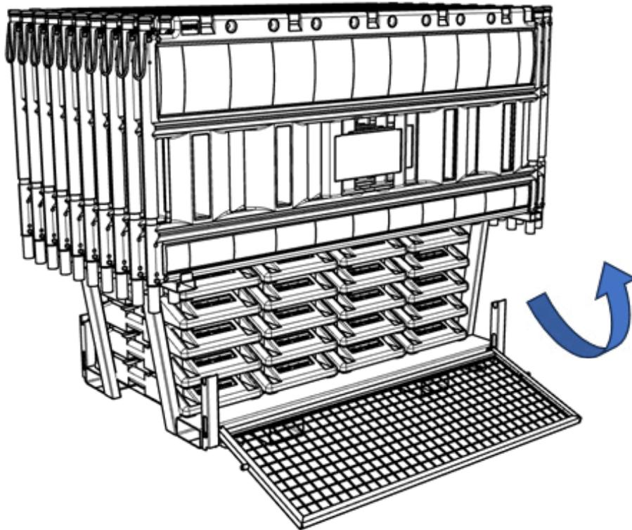
3. Insert the barrier grille into the holes on the rectangular tube on one side.
